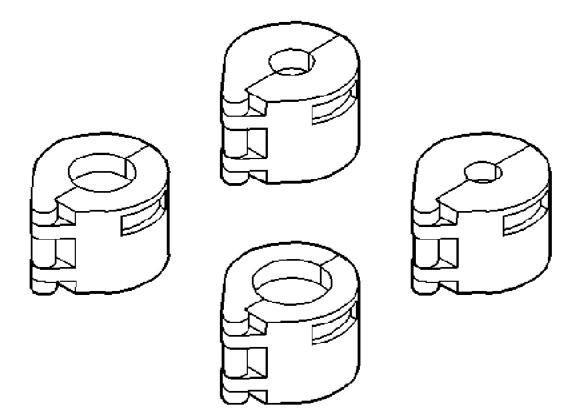
**Fig. 4:** A/C Line Disconnect Tools 7193 Courtesy of CHRYSLER LLC
