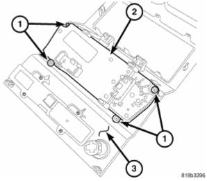
Fig. 43: Removing/Installing Four Screws That Secure A/C-Heater Control To Instrument Panel Center Bezel Courtesy of CHRYSLER LLC
