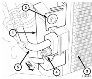
Fig. 139: Radiator, Bolts, A/C Condenser, Nut & A/C Discharge Line Courtesy of CHRYSLER LLC
