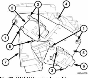
Fig. 77: HVAC Housing Assembly Courtesy of CHRYSLER LLC
