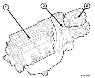
**Fig. 99: Air Distribution Housing, HVAC Housing & Air Inlet Housing Courtesy of CHRYSLER LLC**
