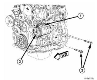
Fig. 124: A/C Clutch Field Coil Connector, Bolts & A/C Compressor Courtesy of CHRYSLER LLC
