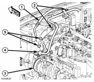
**Fig. 136: Refrigerant Line System** Courtesy of CHRYSLER LLC
