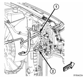
Fig. 141: A/C Liquid Line & Condenser Tube Courtesy of CHRYSLER LLC
