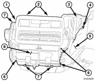
**Fig. 72: Air Distribution Housing Remove/Install Components** Courtesy of CHRYSLER LLC
