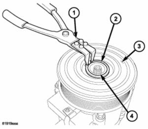
Fig. 24: Using Snap Ring Pliers 9764 Or Equivalent To Remove/Install Snap Ring That Secures Pulley And Bearing Assembly To Front Of A/C Compressor Courtesy of CHRYSLER LLC
