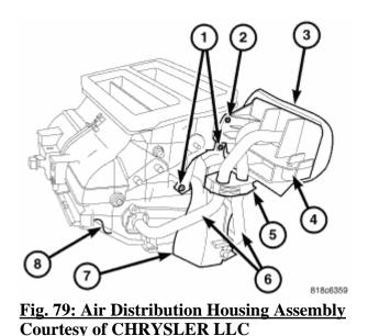
8. Remove the two screws (1) that secure the upper front passenger side floor duct (7) to the passenger side
