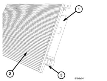
Fig. 200: A/C Receiver/Drier, Left Side A/C Condenser & Bolt Courtesy of CHRYSLER LLC
