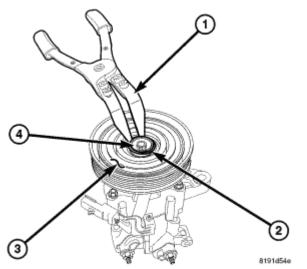
**Fig. 33: Using Snap Ring Pliers To Remove/Install Snap Ring That Secures Pulley And Bearing** <u>Assembly To Front Of A/C Compressor</u> Courtesy of CHRYSLER LLC
