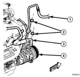
**Fig. 191:** A/C Discharge Line, Nuts, A/C Suction Line & A/C Compressor Courtesy of CHRYSLER LLC
