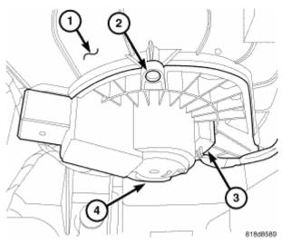
Fig. 113: HVAC Housing, Screws, Instrument Panel Wire Harness Connector & Blower Motor Courtesy of CHRYSLER LLC
