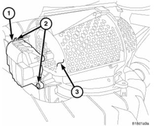
Fig. 18: Recirculation Door Actuator, Screws & Air Inlet Housing
