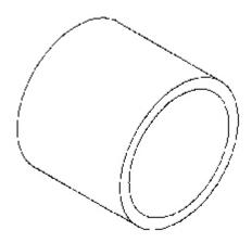
**Fig. 7: Compressor Field Coil Remover 9354** Courtesy of CHRYSLER LLC
