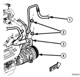
Fig. 188: A/C Discharge Line, Nuts, A/C Suction Line & A/C Compressor Courtesy of CHRYSLER LLC
