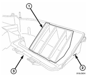
**Fig. 89: Air Deflector Vane, HVAC Housing & Foam Seal Courtesy of CHRYSLER LLC**
