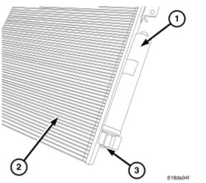
Fig. 199: A/C Receiver/Drier, Left Side A/C Condenser & Bolt Courtesy of CHRYSLER LLC
