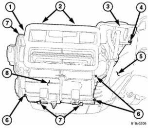
**Fig. 108: Air Distribution Housing Remove/Install Components Courtesy of CHRYSLER LLC**
