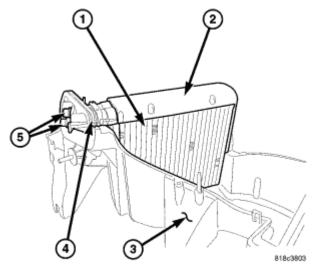
Fig. 95: A/C Evaporator, Foam Insulator, HVAC Housing, Rubber Seal & Tapping Block Courtesy of CHRYSLER LLC
