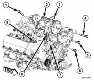
Fig. 130: A/C Compressor Components Courtesy of CHRYSLER LLC
