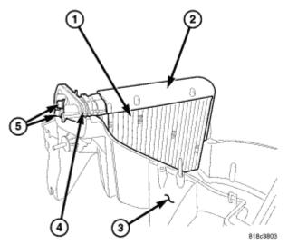
**Fig. 156:** A/C Evaporator, Foam Insulator, HVAC Housing, Rubber Seal & Tapping Block Courtesy of CHRYSLER LLC
