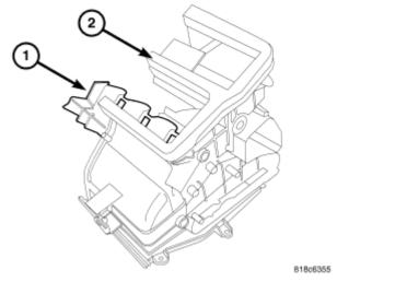
Fig. 82: Air Deflector Vane Assembly & Air Distribution Housing Courtesy of CHRYSLER LLC
