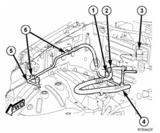
Fig. 174: Removing/Installing LHD Liquid Line Courtesy of CHRYSLER LLC
