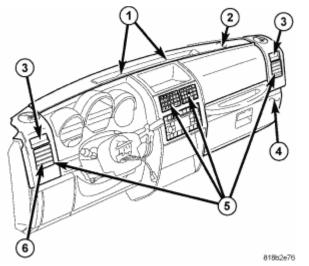
Fig. 115: Defroster Air Outlets, Instrument Panel Top Cover, Side Window Demister Air Outlets, Instrument Panel & Instrument Panel Air Outlets Courtesy of CHRYSLER LLC
