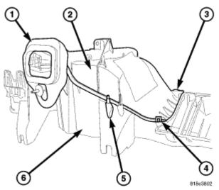
**Fig. 96: Foam Seal, HVAC Housing, Screws, Plastic Retaining Tabs & Metal Clips Courtesy of CHRYSLER LLC**
