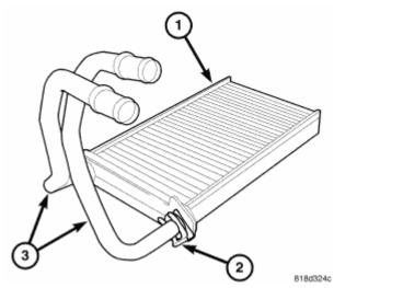
**Fig. 142: Heater Core, Metal Retaining Clamps & Heater Core Tubes** Courtesy of CHRYSLER LLC
