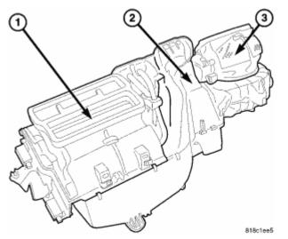
**Fig. 93: Air Distribution Housing, HVAC Housing & Air Inlet Housing Courtesy of CHRYSLER LLC**
