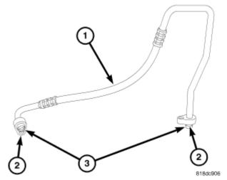
Fig. 157: A/C Discharge Line, Metal Gaskets & Rubber O-Ring Seals Courtesy of CHRYSLER LLC
