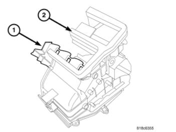
**Fig. 101: Air Deflector Vane Assembly & Air Distribution Housing** Courtesy of CHRYSLER LLC
