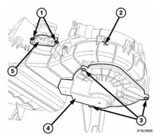
Fig. 85: Screws, HVAC Housing, Blower Motor & Blower Motor Resistor Courtesv of CHRYSLER LLC
