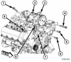
Fig. 129: A/C Compressor Components Courtesy of CHRYSLER LLC
