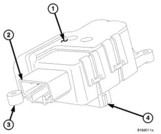
Fig. 13: Identifying Blend Door Actuator, Integral Wire Connector Receptacle, Integral Mounting Tabs <u>& Output Shaft</u> Courtesy of CHRYSLER LLC
