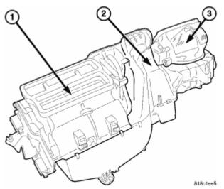
Fig. 90: Air Distribution Housing, HVAC Housing & Air Inlet Housing Courtesy of CHRYSLER LLC
