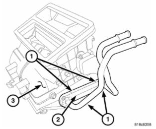
**Fig. 145: Plastic Retaining Tabs, Heater Core & Air Distribution Housing Courtesy of CHRYSLER LLC**
