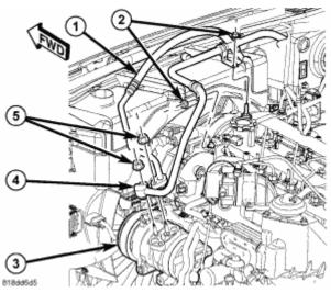
**Fig. 197: Refrigerant Line System** Courtesy of CHRYSLER LLC
