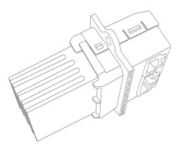
**Fig. 44: Power-Blower Motor Module** Courtesy of CHRYSLER LLC
