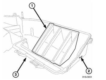
**Fig. 94: Air Deflector Vane, HVAC Housing & Foam Seal Courtesy of CHRYSLER LLC**
