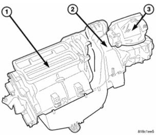
Fig. 84: Air Distribution Housing, HVAC Housing & Air Inlet Housing Courtesy of CHRYSLER LLC
