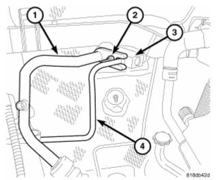
Fig. 196: A/C Suction Line, Nut, A/C Expansion Valve & A/C Liquid Line Courtesy of CHRYSLER LLC
