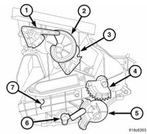
Fig. 78: Removing/Installing Defrost Door Lever/Gear Assembly, Mode Door Cam, Panel Door Gear, Blend Door Gear, Blend Door Lever And Blend Door Cam From Driver Side Of Air Distribution Housing Courtesy of CHRYSLER LLC
