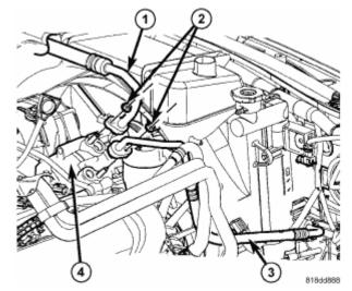
Fig. 195: Removing/Installing Nuts That Secure A/C Suction Line And A/C Discharge Line To A/C
