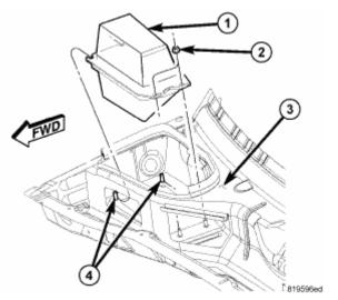
Fig. 73: Air Inlet Screen, Nuts, Cowl Panel & Retaining Studs Courtesy of CHRYSLER LLC
