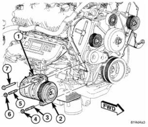
**Fig. 132: Removing/Installing A/C Compressor** Courtesy of CHRYSLER LLC
