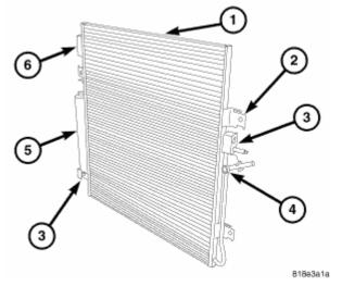
Fig. 137: A/C Condenser Components Courtesy of CHRYSLER LLC
