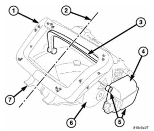
Fig. 91: Foam Seal, Parting Line, Recirculation-Air Door, Recirculation Door Actuator, Screws & <u>Air Inlet Housing</u> Courtesy of CHRYSLER LLC
