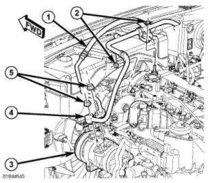
**Fig. 182: Refrigerant Line System** Courtesy of CHRYSLER LLC
