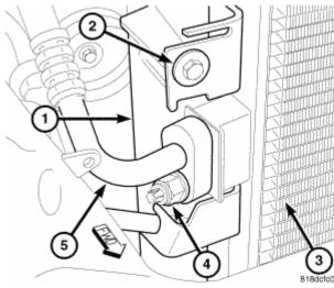
Fig. 140: Radiator, Bolts, A/C Condenser, Nut & A/C Discharge Line Courtesy of CHRYSLER LLC
