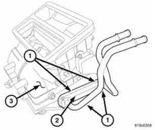
Fig. 144: Plastic Retaining Tabs, Heater Core & Air Distribution Housing Courtesy of CHRYSLER LLC
