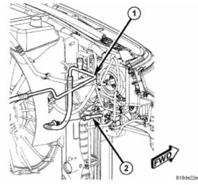
Fig. 171: A/C Liquid Line & Condenser Tube Courtesy of CHRYSLER LLC
