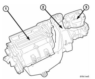
Fig. 71: Air Distribution Housing, HVAC Housing & Air Inlet Housing Courtesy of CHRYSLER LLC
