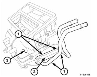
**Fig. 80: Plastic Retaining Tabs, Heater Core & Air Distribution Housing Courtesy of CHRYSLER LLC**
