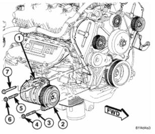
**Fig. 127: Removing/Installing A/C Compressor** Courtesy of CHRYSLER LLC
