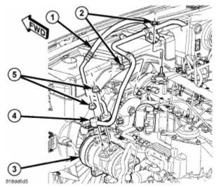
**Fig. 123: Refrigerant Line System** Courtesy of CHRYSLER LLC
