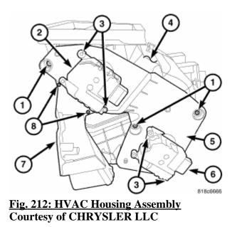
4. Install the driver side front floor duct (7) onto the driver side of the air distribution housing (4) and install the retaining screw (8). Tighten the screw to 1.2 N.m (10 in lbs.).
