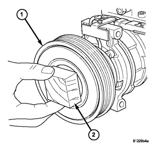
**Fig. 36: Installing Pulley And Bearing Assembly Onto Front Of A/C Compressor Courtesy of CHRYSLER LLC**
