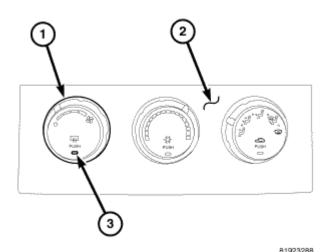
Fig. 2: Identifying Push-Button Switch & A/C-Heater Control Courtesy of CHRYSLER LLC
