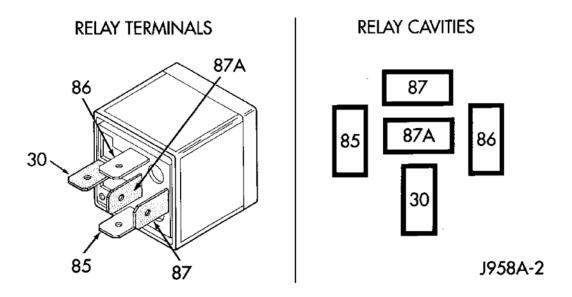
Fig. 5: Rear Window Defogger Relay Courtesy of CHRYSLER LLC
