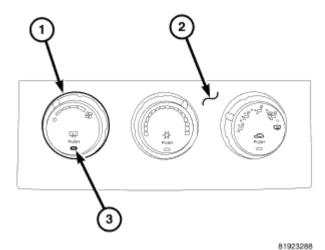
Fig. 8: Identifying Push-Button Switch & A/C-Heater Control Courtesy of CHRYSLER LLC
