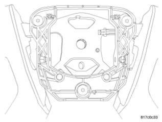
Fig. 2: Horn Switch Courtesy of CHRYSLER LLC
