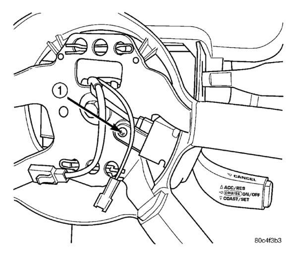
Fig. 3: Speed Control Switch Mounting Screws Courtesy of CHRYSLER LLC
