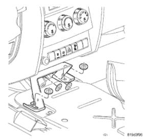
Fig. 316: Removing/Installing Nuts And Instrument Panel Support Bracket Courtesy of CHRYSLER LLC
