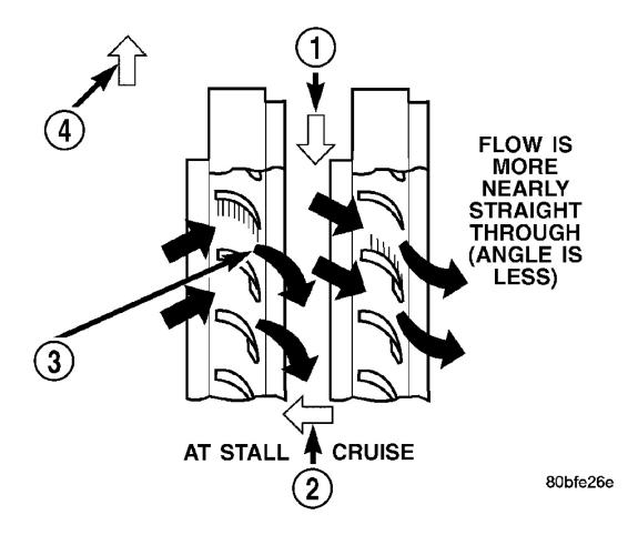
Fig. 274: Stator Operation Courtesy of CHRYSLER LLC
