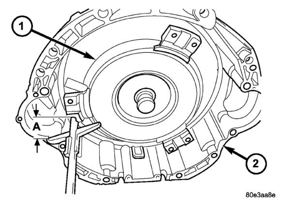
Fig. 276: Measuring Torque Converter Installation Depth Courtesy of CHRYSLER LLC
