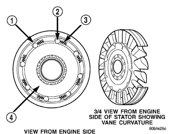
Fig. 270: Stator Components
