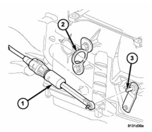
Fig. 67: Connecting Gearshift Cable To Support Bracket And Transmission Manual Lever Courtesy of CHRYSLER LLC
