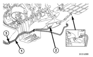
**Fig. 69: Connecting Cooler Lines Into Transmission** Courtesy of CHRYSLER LLC
