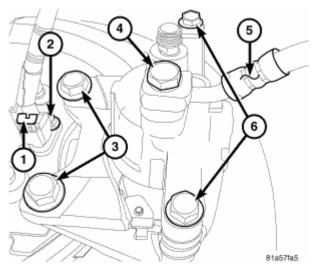
**Fig. 20: Identifying Bolts, Brake Hose & Brake Hose Banjo Bolt** Courtesy of CHRYSLER LLC
