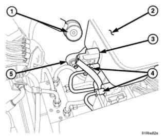
Fig. 58: Identifying Reservoir, Fluid Level Electrical Connector, Brake Lines, Mounting Nuts & Booster Check Valve Courtesy of CHRYSLER LLC
