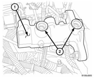
**Fig. 73: Identifying Old Grommets & Cylinder Body Courtesy of CHRYSLER LLC**
