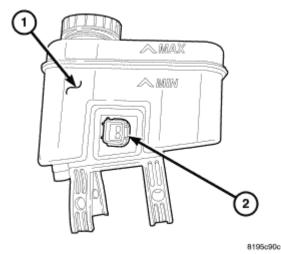
**Fig. 77: Identifying Master Cylinder Reservoir Courtesy of CHRYSLER LLC**
