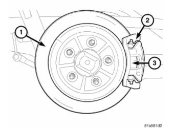
Fig. 42: Rear Disc Brake Rotor Courtesy of CHRYSLER LLC
