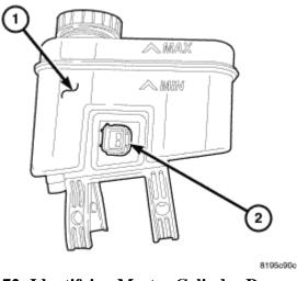
**Fig. 72: Identifying Master Cylinder Reservoir Courtesy of CHRYSLER LLC**
