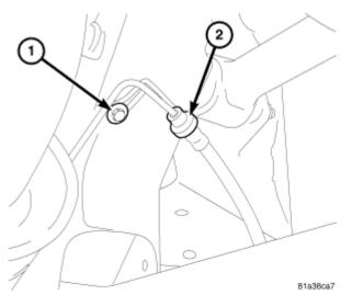
Fig. 9: Identifying Brake Hose/Line Mounting Bolt & Line/Hose Courtesy of CHRYSLER LLC
