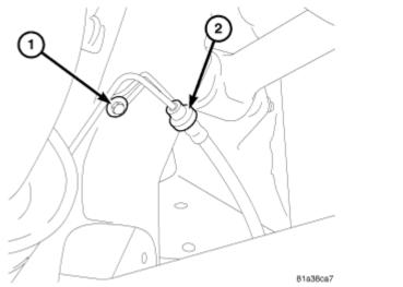
Fig. 6: Identifying Brake Hose/Line Mounting Bolt & Line/Hose Courtesy of CHRYSLER LLC
