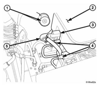
Fig. 68: Identifying Reservoir, Fluid Level Electrical Connector, Brake Lines, Mounting Nuts & Booster Check Valve Courtesy of CHRYSLER LLC
