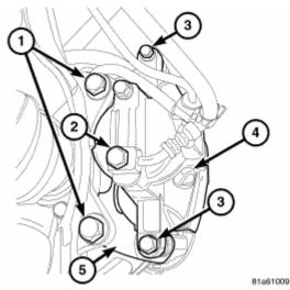
Fig. 21: Disc Brake Caliper Components Courtesy of CHRYSLER LLC
