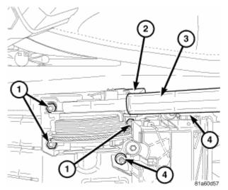
Fig. 91: Identifying Parking Brake Lever Assembly Mounting Nuts, Parking Brake Lamp Switch Wire,
