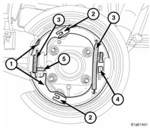
**Fig. 94: Identifying Brake Shoes Courtesy of CHRYSLER LLC**
