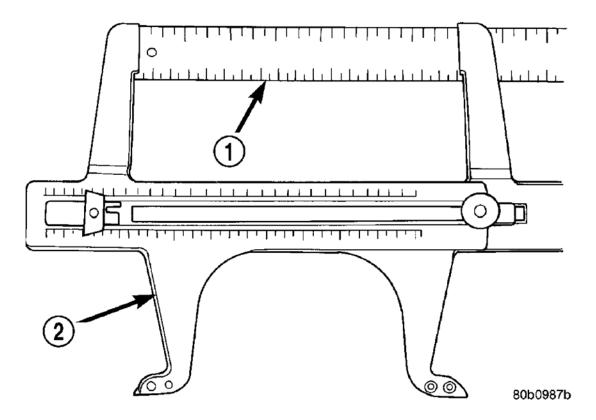
**Fig. 100: Setting Gauge To Park Brake Shoe Measurement** Courtesy of CHRYSLER LLC
