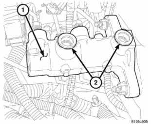
**Fig. 74: Identifying Old Grommets & Cylinder Body** Courtesy of CHRYSLER LLC
