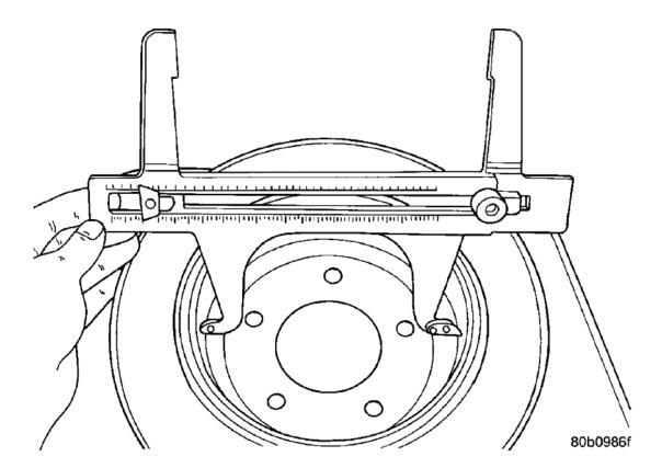
**Fig. 98: Measuring Park Brake Drum Diameter** Courtesy of CHRYSLER LLC
