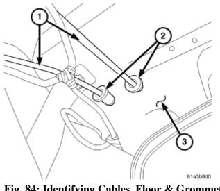
**Fig. 84: Identifying Cables, Floor & Grommets Courtesy of CHRYSLER LLC**
