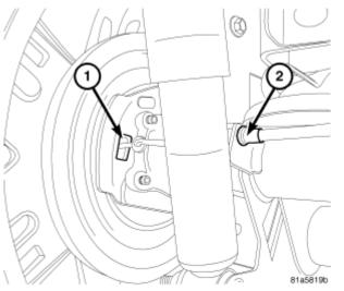
**Fig. 86: Identifying Brake Lever & Brake Cable** Courtesy of CHRYSLER LLC
