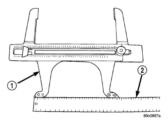
**Fig. 99: Reading Park Brake Drum Diameter** Courtesy of CHRYSLER LLC
