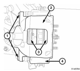
Fig. 15: Identifying Caliper Mounting Bolts, Disc Brake Caliper, Inboard/Outboard Pads & Adapter
