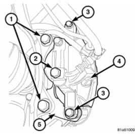
Fig. 36: Disc Brake Caliper Components Courtesy of CHRYSLER LLC
