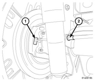
**Fig. 85: Identifying Brake Lever & Brake Cable** Courtesy of CHRYSLER LLC
