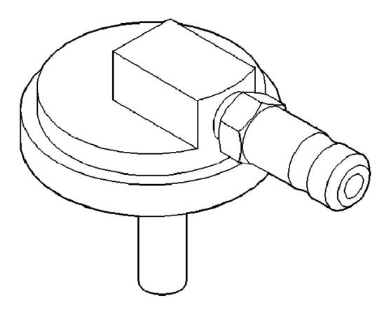
**Fig. 4: Adapter Pressure Bleeder 6921** Courtesy of CHRYSLER LLC
