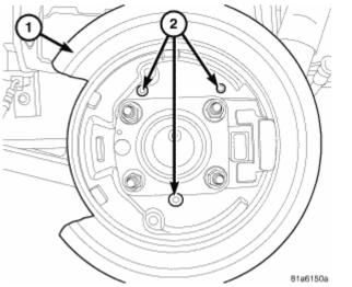
**Fig. 80: Identifying Support Plate & Attaching Bolts** Courtesy of CHRYSLER LLC
