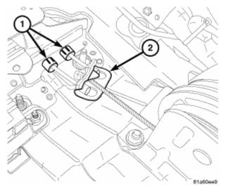
**Fig. 83: Identifying Cables & Equalizer** Courtesy of CHRYSLER LLC
