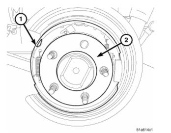
Fig. 97: Identifying Rear Park Brake Shoes & Axle Shaft Courtesy of CHRYSLER LLC
