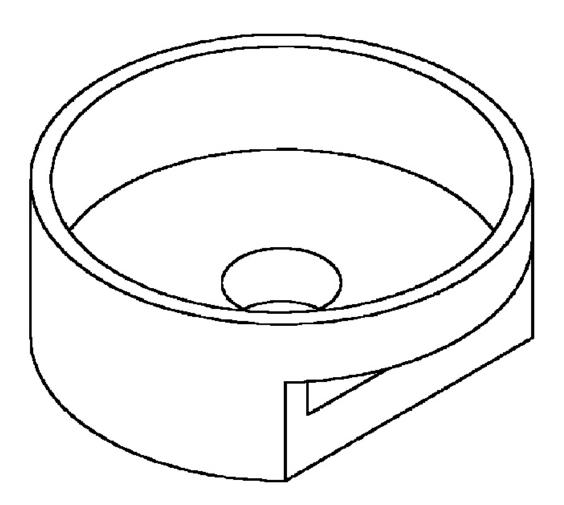
**Fig. 2: Installer Caliper Dust Boot 8280** Courtesy of CHRYSLER LLC
