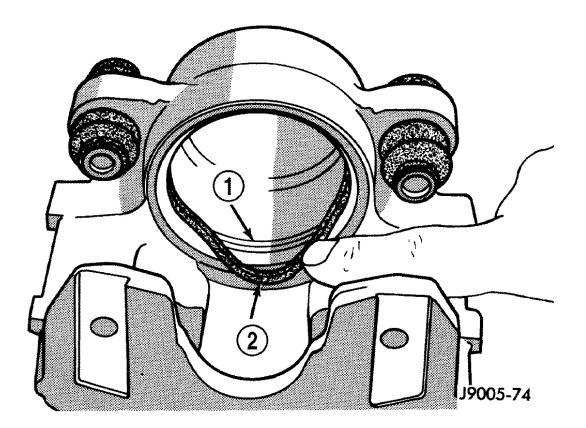
**Fig. 29: Installing Piston Seal - Typical Courtesy of CHRYSLER LLC**
