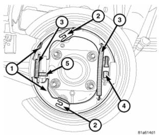
**Fig. 96: Identifying Brake Shoes** Courtesy of CHRYSLER LLC
