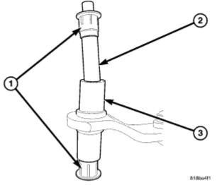
**Fig. 47: Pedal Bushing** Courtesy of CHRYSLER LLC
