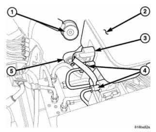
Fig. 70: Identifying Reservoir, Fluid Level Electrical Connector, Brake Lines, Mounting Nuts & Booster Check Valve
