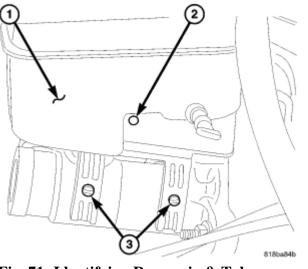
**Fig. 71: Identifying Reservoir & Tabs Courtesy of CHRYSLER LLC**
