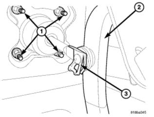
**Fig. 48: Identifying Retainer Clip, Pedal & Booster Mounting Nuts** Courtesy of CHRYSLER LLC
