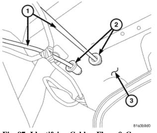
**Fig. 87: Identifying Cables, Floor & Grommets Courtesy of CHRYSLER LLC**
