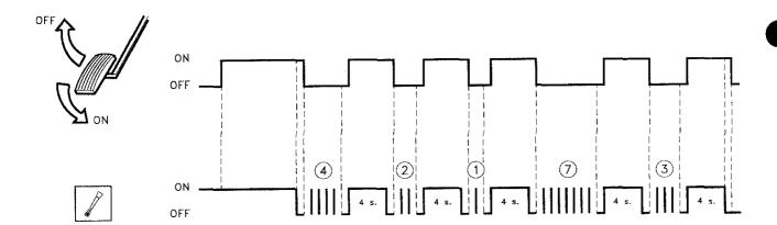
NOTE: If this procedure is not activated correctly, check the throttle potentiometer and the corresponding wiring, and also the throttle itself (throttle stroke without obstacles or sticking); also check the supply to the C.C.M..
