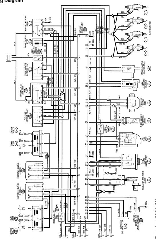
(\*) up to chassis N.31212 = 7.5A from chassis N.31213 = 15.A (\*\*) from chassis N.....
